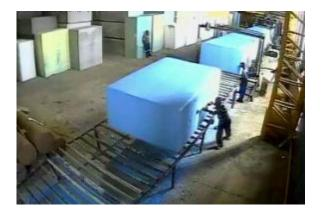
This machine can be used for continuous producing Flexible Polyurethane Foam(maxfoam), which density is 9~50KGS/M³. It can be automatic cutting the foam into difference sizes which is according to client's requirement. It can be realized numerical control with accurate and convenient ration during the whole production. It becomes more easily and stable to operate the machine.
